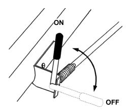
In the "ON" position, the material exiting the right hand side is deflected as shown. This allows the spreader to be butted up against a sidewalk, driveway, lot line etc. minimizing the amount of material thrown into these areas.
