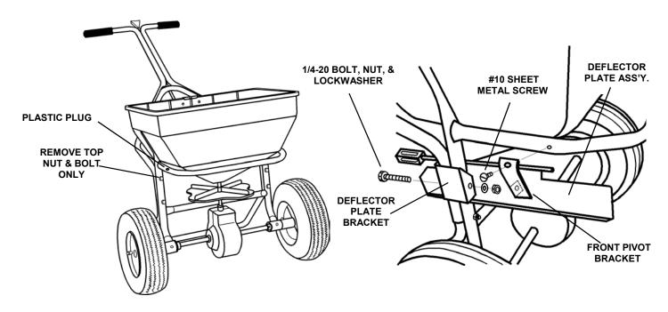
**2.** With Deflector Plate in the "**DOWN**" position, Insert the longer end of the Control Rod with the formed tab into the slotted bracket on the Deflector Plate assembly as shown. Rotate the rod as shown to secure rod into bracket.
