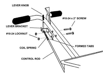
**3.** Slide the Coil Spring onto Rod until it touches the formed tabs on Control Rod, followed by the Lever Bracket as shown. Align holes in side of Upper Handle and the Lever Bracket and secure with two (2) #10-24 x 2" stainless steel screws and locknuts supplied. Slide Lever Knob on end of Rod.
